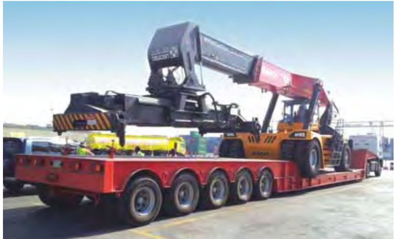
The new low bed trailer has 5 axles of 16 tons per axle and has 20 tires. It has a load floor and 10 meters in addition to the possibility of loading in the area of the axles.
